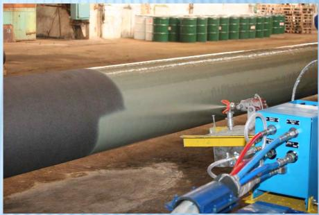
Pipe insulation in the factory and semi-stationary conditions
